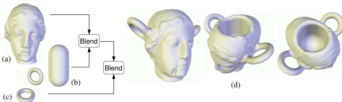
Figure 8. Creating a bowl from the Igea mesh: (a) the original Igea mesh, carved using a negative potential field generated by a line segment implicit primitive (b); (c) the handles created from two implicit circle primitives which are locally blended with the head using an implicit box so as to obtain the final model in (d).
